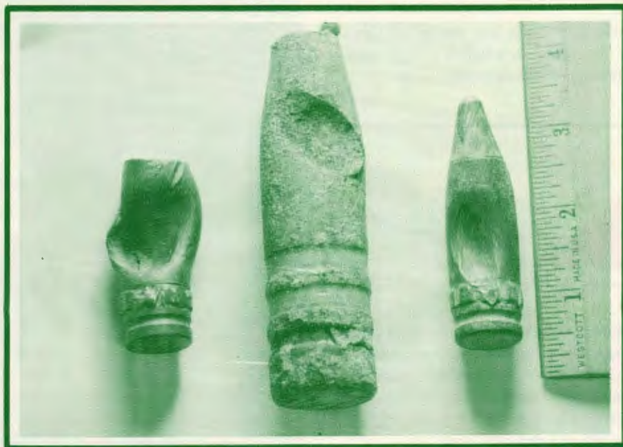
Strafe Pit Debris —A 30mm and two 20mm rounds policed out of a strafe pit. They've all been hit by another round. Notice that the 30mm round has a 20mm-sized groove in it.
